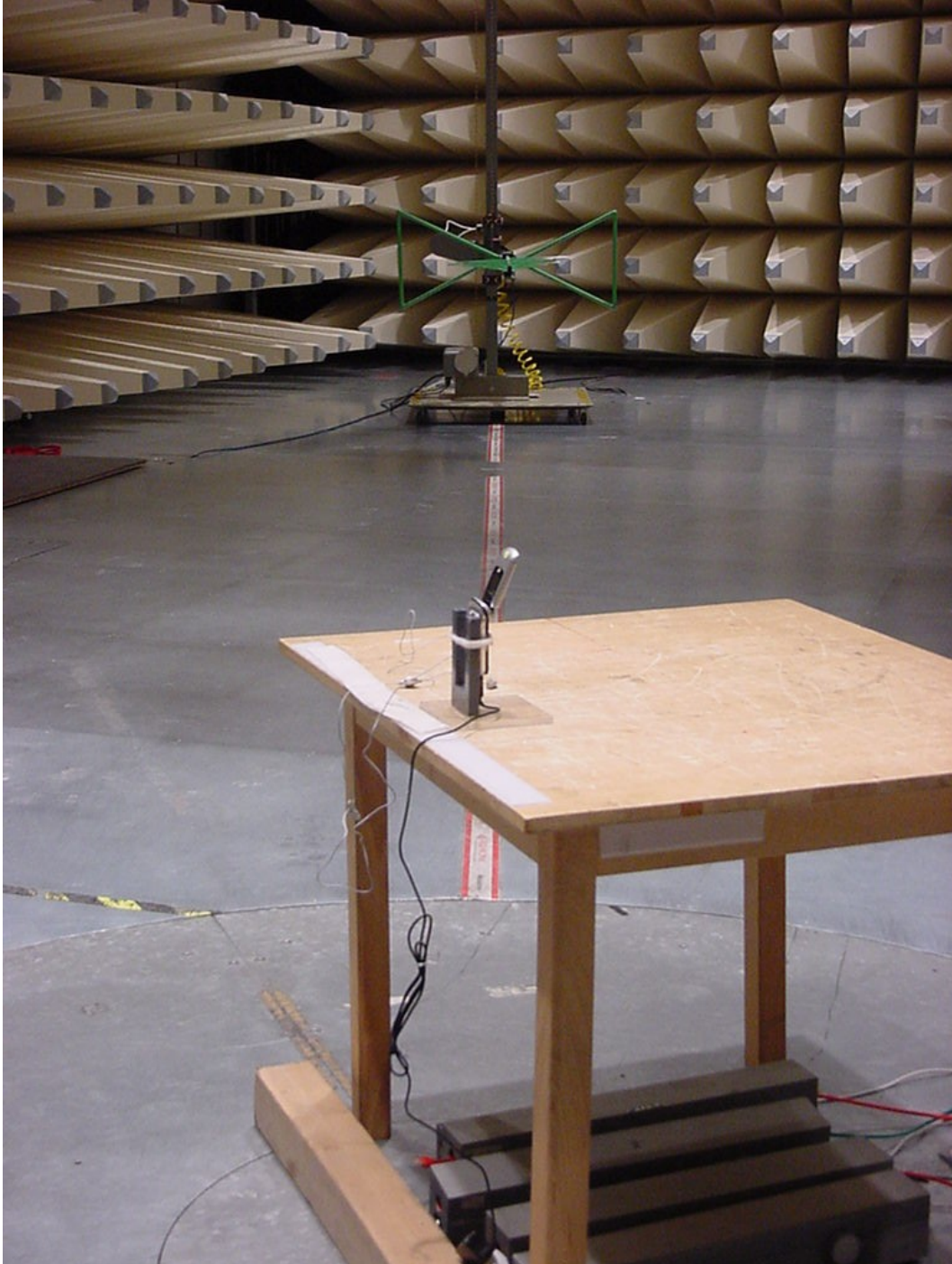
Photo 2 (Radiated Emissions): Test set-up I
