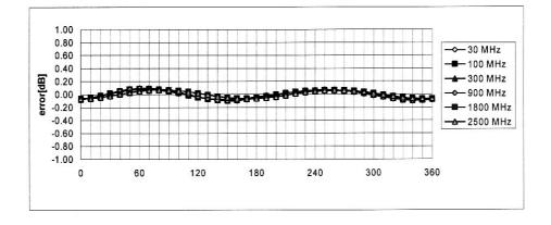
Axial Isotropy Error < ± 0.2 dB
