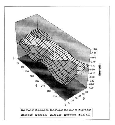
Spherical Isotropy Error < ± 0.4 dB
