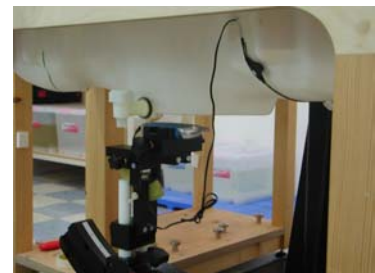
Fig. 18. Body SAR Test Setup with Holster
