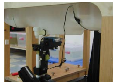
Fig. 19. Body SAR Test Setup with Holster
