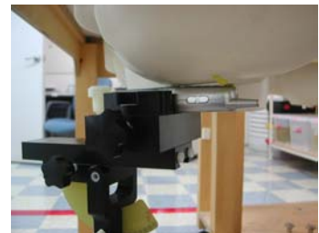
Fig. 17. Head SAR Test Setup
