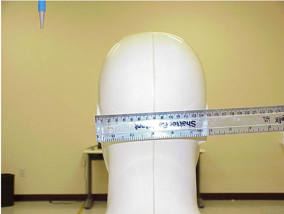
Photo 15. Photo to demonstrate 15 cm Z-axis head phantom
