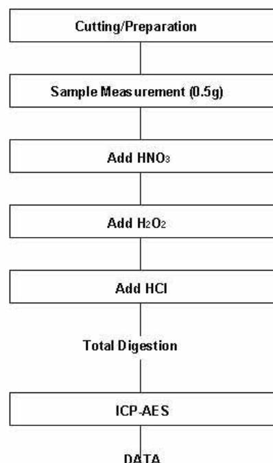
The samples were dissolved totally by pre-conditioning method according to above flow chart.
