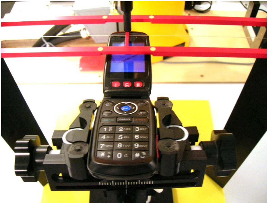
Figure 17-2 HAC Phantom Plane Alignment
