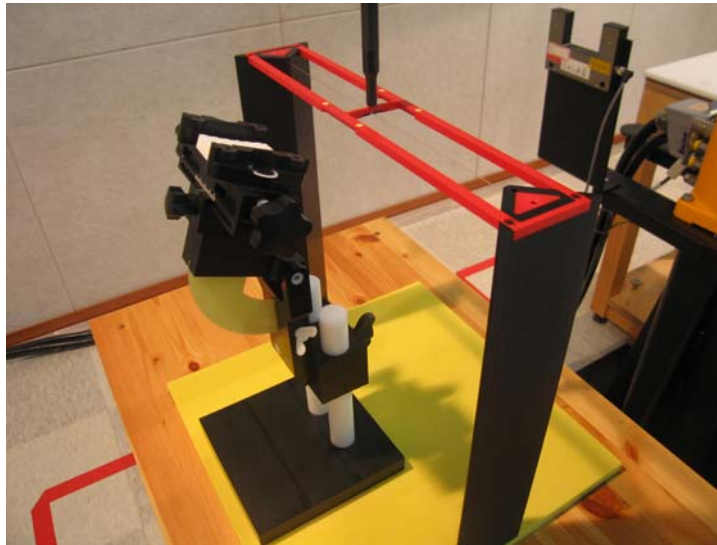
Figure 2. HAC Phantom & Device Holder
