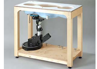
Fig. 8 Generic Twin Phantom
