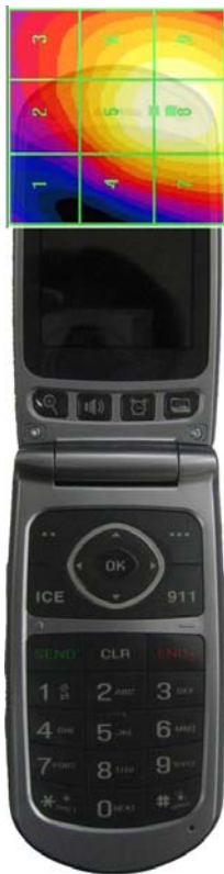
GSM E-Field WD Scan overlay
