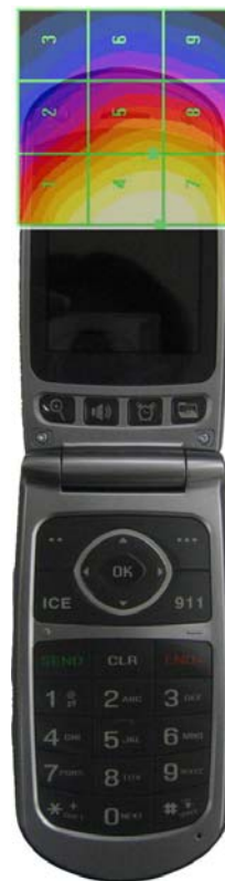
GSM H-Field WD Scan overlay
