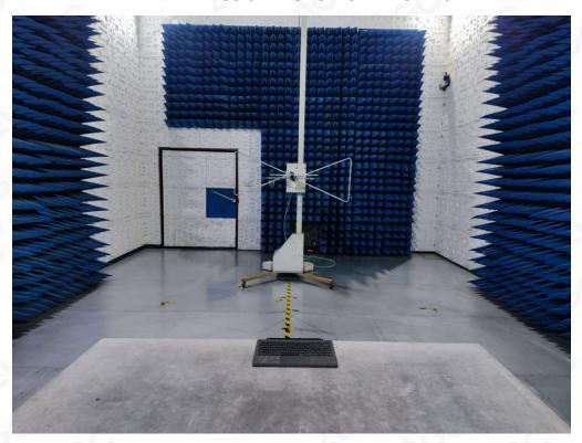
RADIATED EMISSION TEST SETUP ABOVE 1GHz
