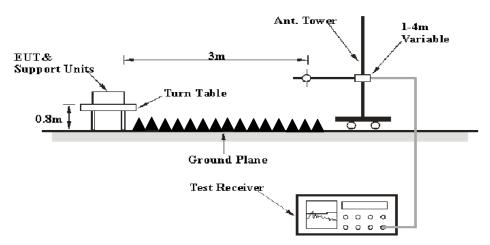
The radiated emission tests were performed in the 3 meters test site, using the setup accordance with the ANSI C63.4-2003. The specification used was the FCC 15.209, and FCC 15.247 limits.
