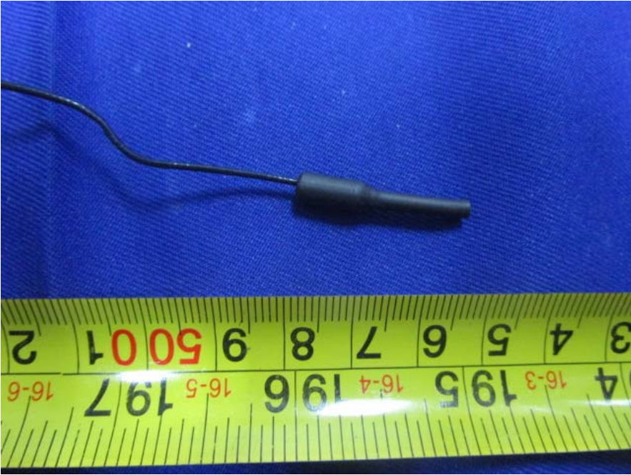
EUT –RF Antenna View
