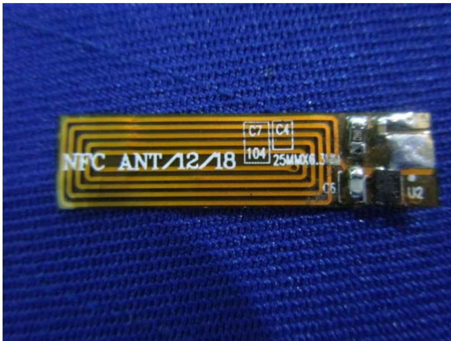
EUT – NFC Board Top View
