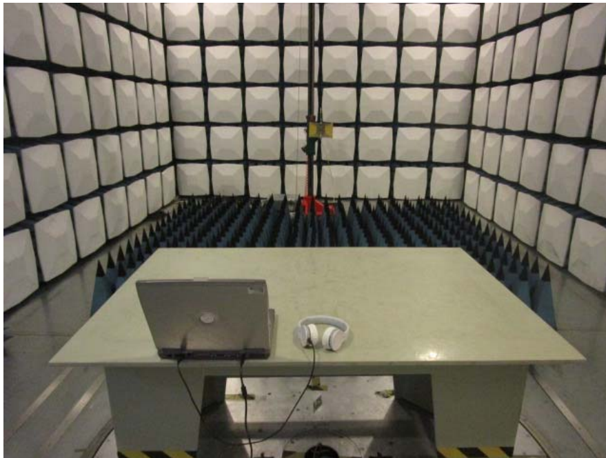
Radiated Emission - Above 1GHz –Rear View
