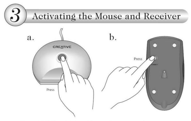
Press the button on the receiver first and then press the button on the mouse to activate the mouse.
