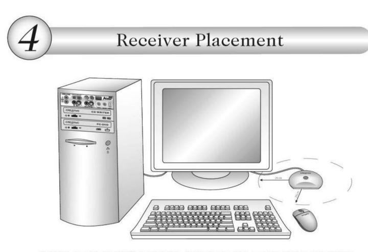
Place the receiver at least 20 cm away from the mouse or other electrical devices, such as your computer and computer monitor, for optimal performance. (Maximum operating range: 1.5 meters)
