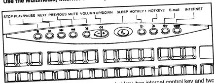
You can find 7 multimedia key ,1 power control key, two internet control key and two Programmable hotkeys at your cordless keyboard., which can control you computer Or access application program in one touch.
