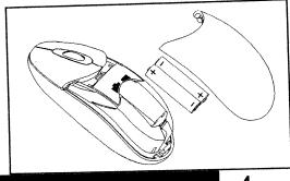
For normal use, two AAA size Alkaline battery can be used up to 6 months. Alkaline Batteries is recommended for both keyboard and mouse.
