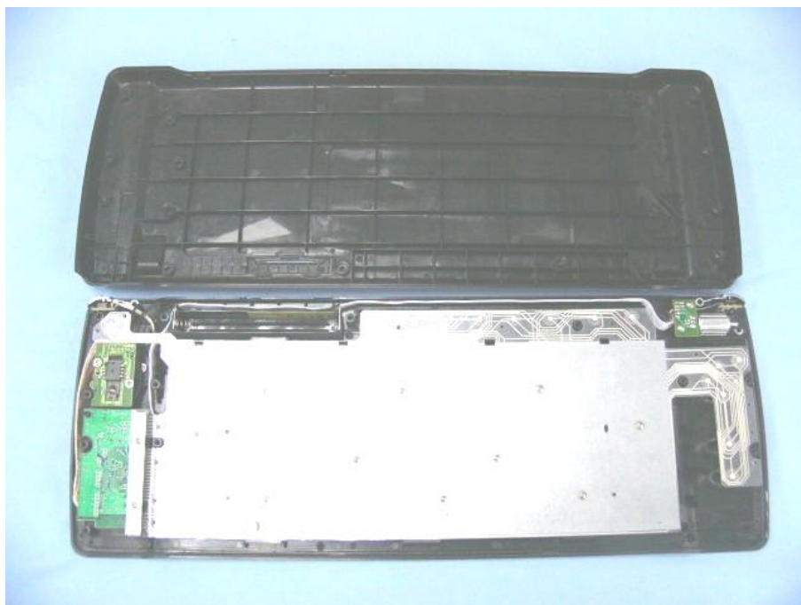
Main & RF board component side
