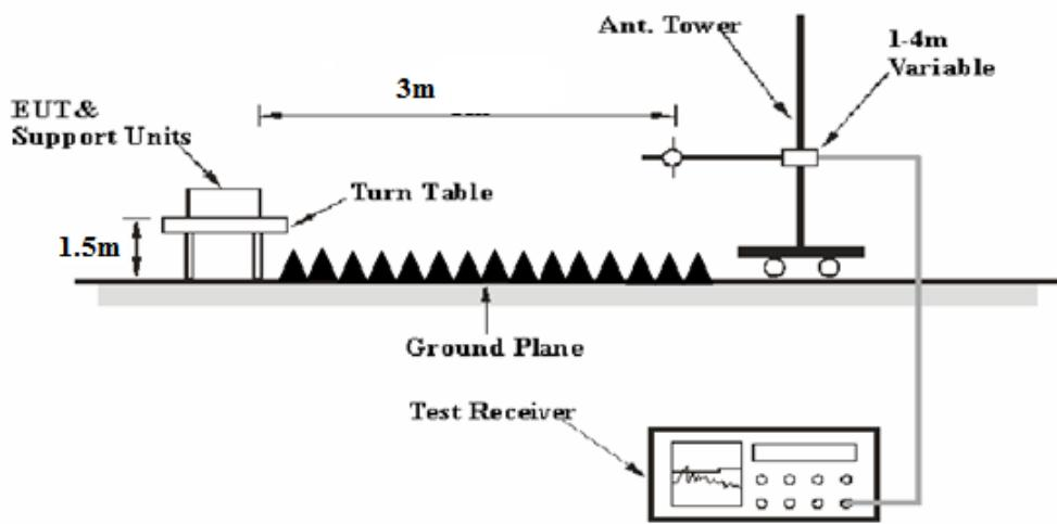
The radiated emission tests were performed in the 3 meters distance, using the setup accordance with the ANSI C63.10-2013. The specification used was the FCC 15.209/15.205 and FCC 15.249 limits.
