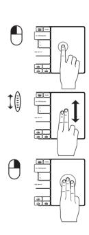
The touch pad could be used as number keyboard or mouse touchpad, transform between them by finger sliding on the slide bar.
