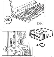
Plug receiver into Usb port. The receiver will match the keyboard automatically.
