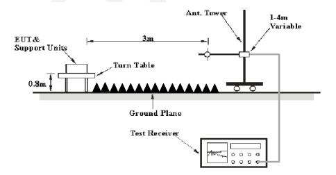
The radiated emission and out of band emission tests were performed in the 3 meters chamber test site, using the setup accordance with the ANSI C63.4-2009. The specification used was the FCC 15.209/15.205 and FCC 15.249 limits.
