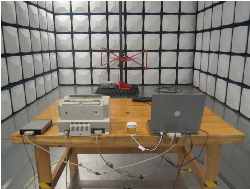
Radiated Emission - Below 1GHz Rear View
