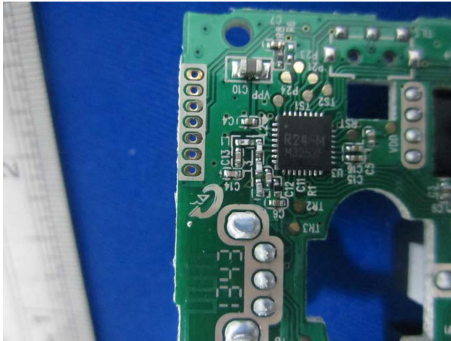
EUT –RF Chip View
