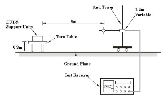
The radiated emission and out of band emission tests were performed in the 3 meters chamber test site, using the setup accordance with the ANSI C63.4-2009. The specification used was the FCC 15.209/15.205 and FCC 15.249 limits.
