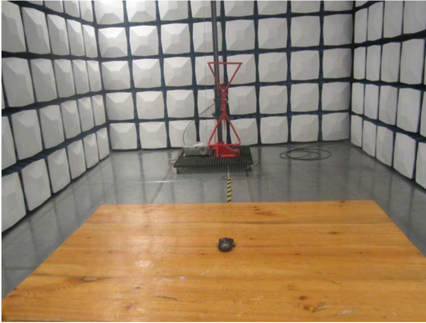
Radiated Emissions Below 1G View
