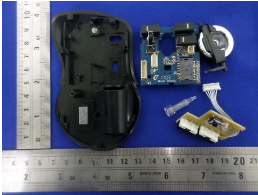
EUT – Cover Off View
