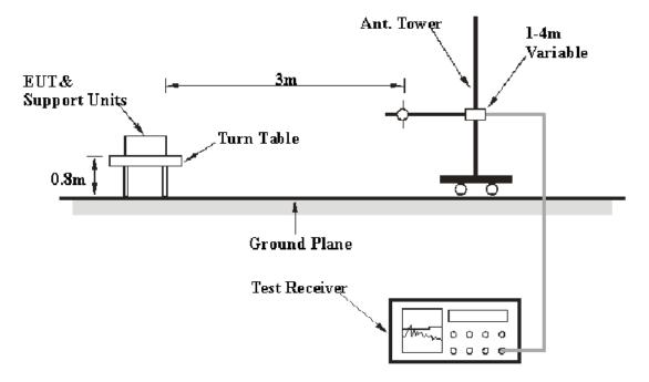
The radiated emission and out of band emission tests were performed in the 3 meters chamber test site, using the setup accordance with the ANSI C63.4-2009. The specification used was the FCC 15.209/15.205 and FCC 15.249 limits.
