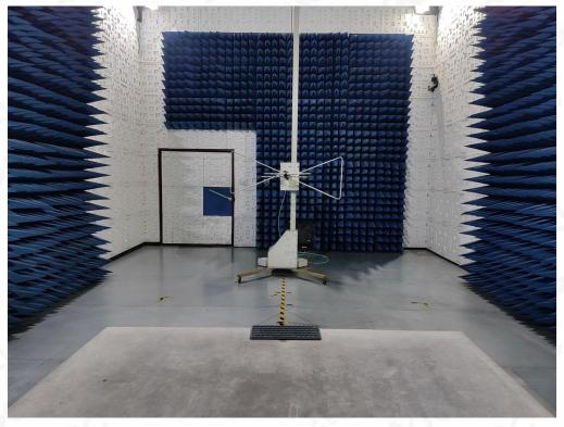
RADIATED EMISSION TEST SETUP ABOVE 1GHz
