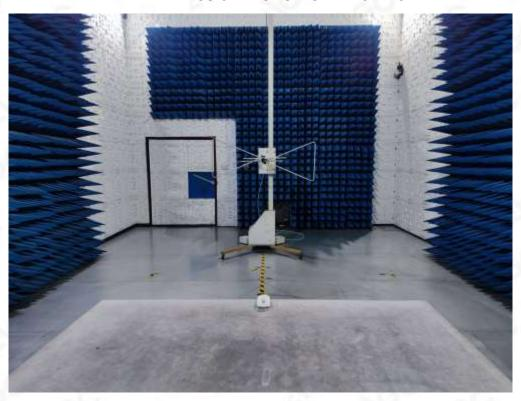
RADIATED EMISSION TEST SETUP ABOVE 1GHz
