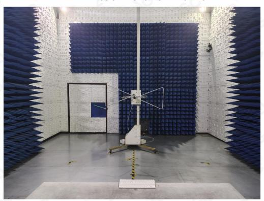
RADIATED EMISSION TEST SETUP ABOVE 1GHz
