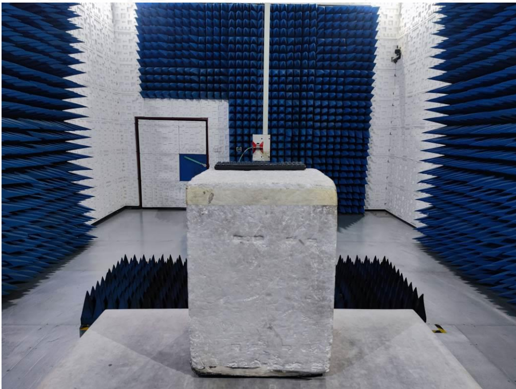
RADIATED EMISSION TEST SETUP ABOVE 1GHZ
