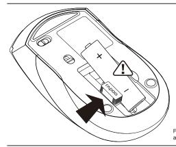
Plug the receiver into the usb port. The receiver will pair with the mouse/keboard automatically.
