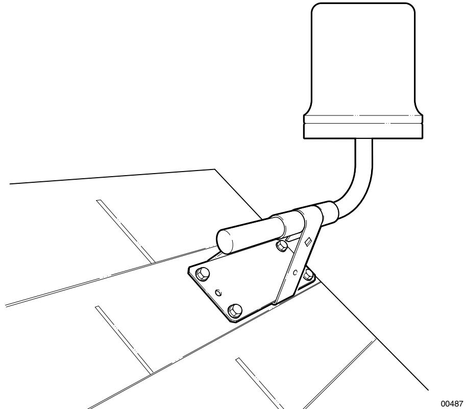
When installing the ERU on a roof, install it in the highest possible location to maximize the signal you receive.
