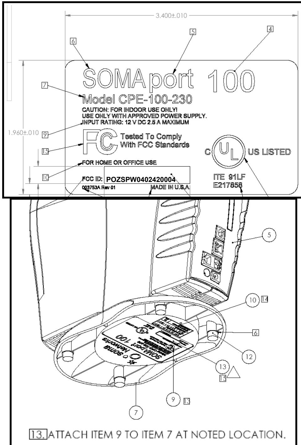
**NOTE:** INFORMATION FOR LABEL DWG IS FROM DWG. NO. 003753A REV 01, LABEL, REGULATORY, U.S.A., SP, WCS, [SOMAPORT 100, MODEL CPE-100-230], NTERIM. LABEL PLACEMENT INFORMATION WAS EXTRACTED FROM DRAWING NUMBER AD-100001-000, ASSY DWG MX, SYSTEM, SP, 2-LINE, REV 02.
