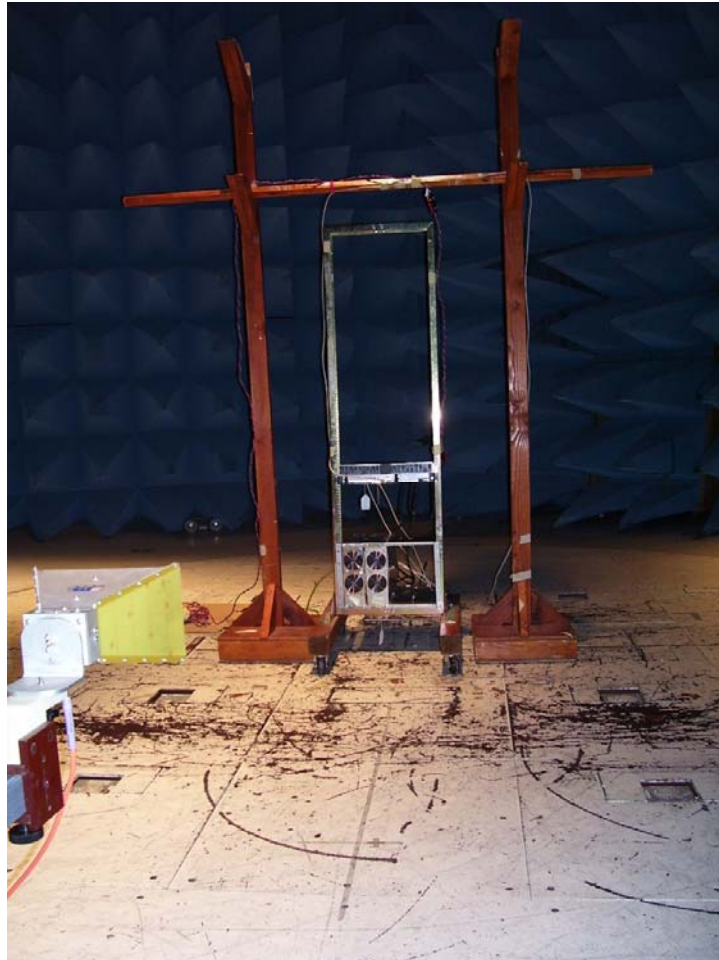
Photograph 3. Radiated Emissions Test Setup
