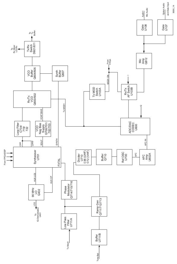
Figure 3-3 VHF/UHF Synthesiser, Block Diagram
