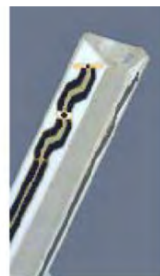
Figure 2.3 Probe Thick-Film Technique
