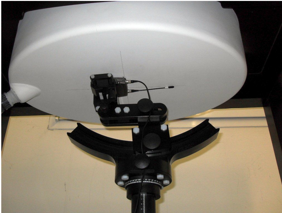
Figure 3 – Tested Device position: with the back side against the phantom (detail)
