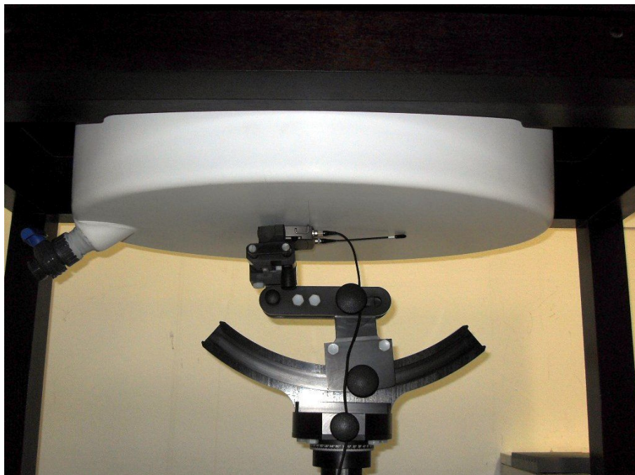
Figure 2 – Tested Device position: with the back side against the phantom
