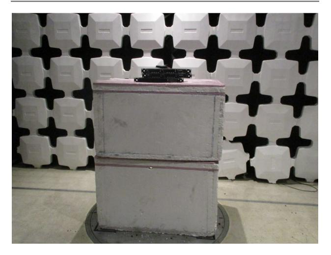
Radiated Testing, Below 1 GHz
