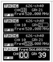
In this menu channel/group and frequencies can be setup. The name of the group is shown on the top right of the display. SYNC group is a quick self-settable channel synchronized by receiver (with SYNC group, on the top right of the display is shown the name of the synchronized receiver).
