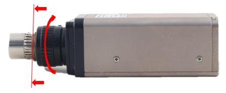
**WARNING:** for a correct insertion of the microphone/boom, **screw the ferrule up to the end of the threading** and then connect the mic/boom.
