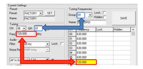
Using the LOAD/SAVE button, at the bottom of the panel, it is possible to **load/save** the frequencies for the selected group from/to a .wdf file. To save the frequencies of all the groups click to the related button above. The legacy option save the channels without the hidden/lock info.
