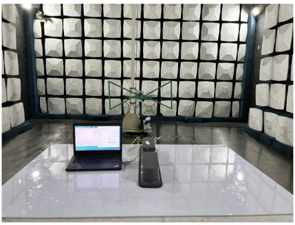
**Radiated Test Above 1GHz**
