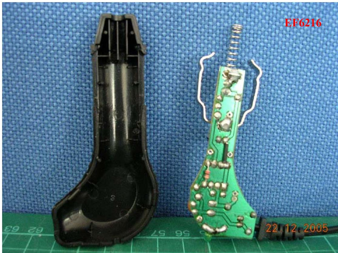
**Photo 7: Internal photo of vehicle charger**
