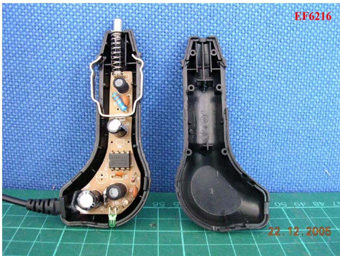
**Photo 6: Internal photo of vehicle charger**
