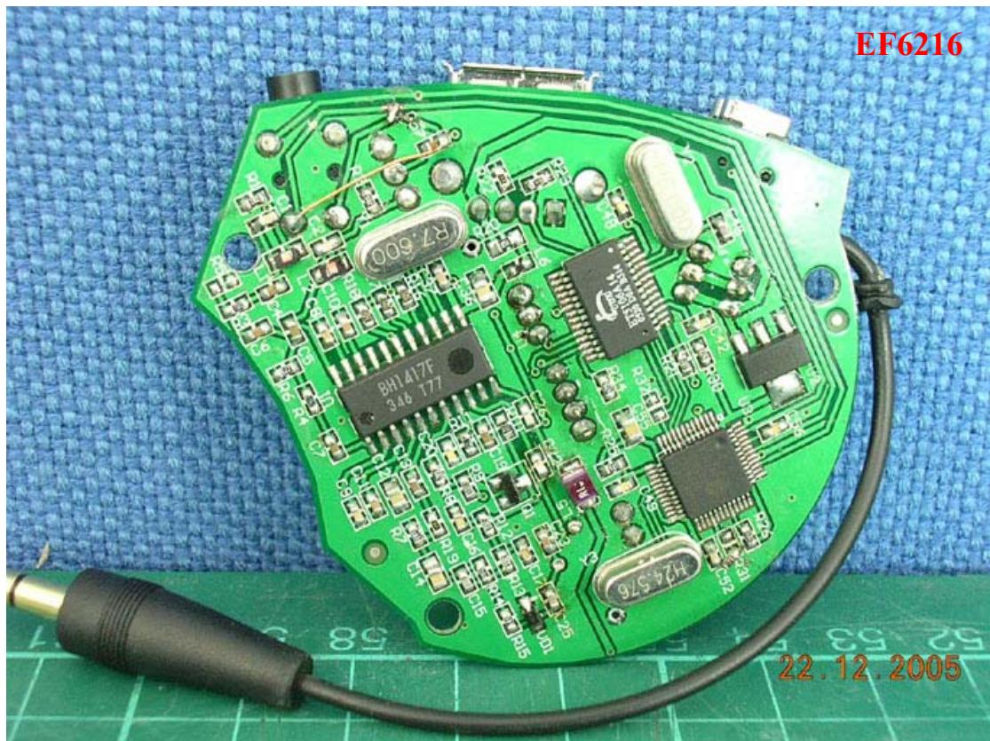
**Photo 5: Internal photo of vehicle charger**
