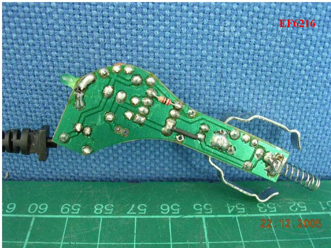
**Photo 8: Internal photo of vehicle charger**
