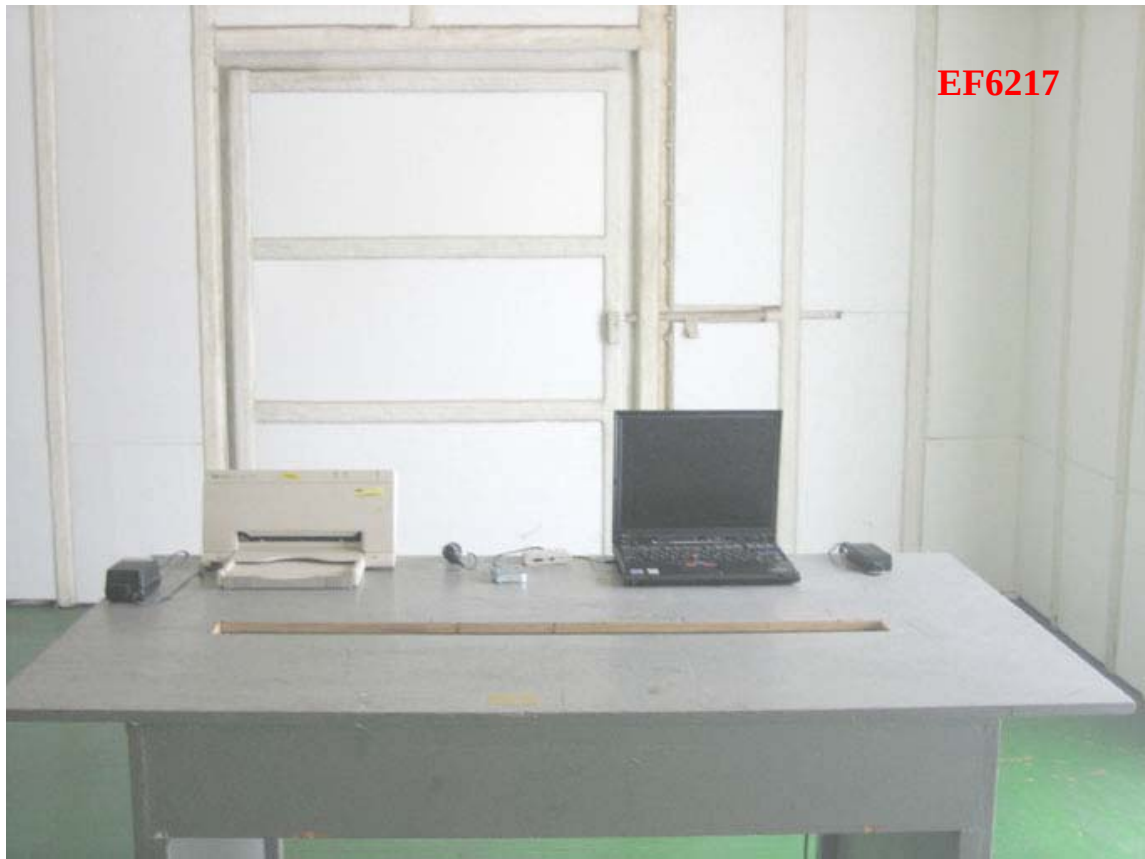
Photo 1: Spurious Emission Test Set-up photo
