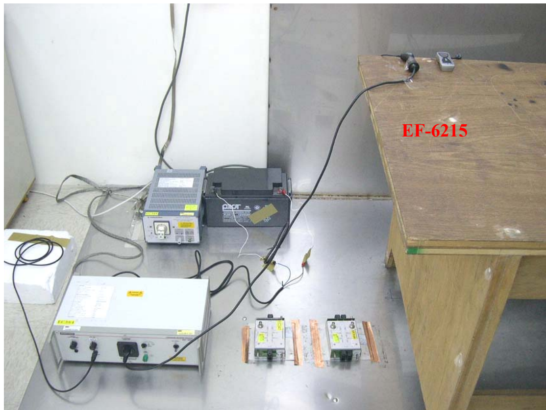
Photo 1: Conducted Emission Test Set-up
