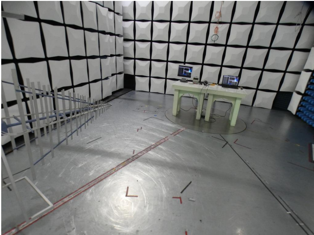
Photo 1: Test setup for radiated measurements FCC15b, below 1 GHz
