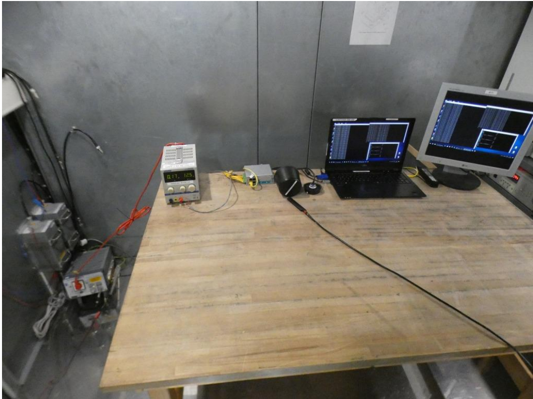
Photo 4: Test setup for conducted measurements FCC15b.
