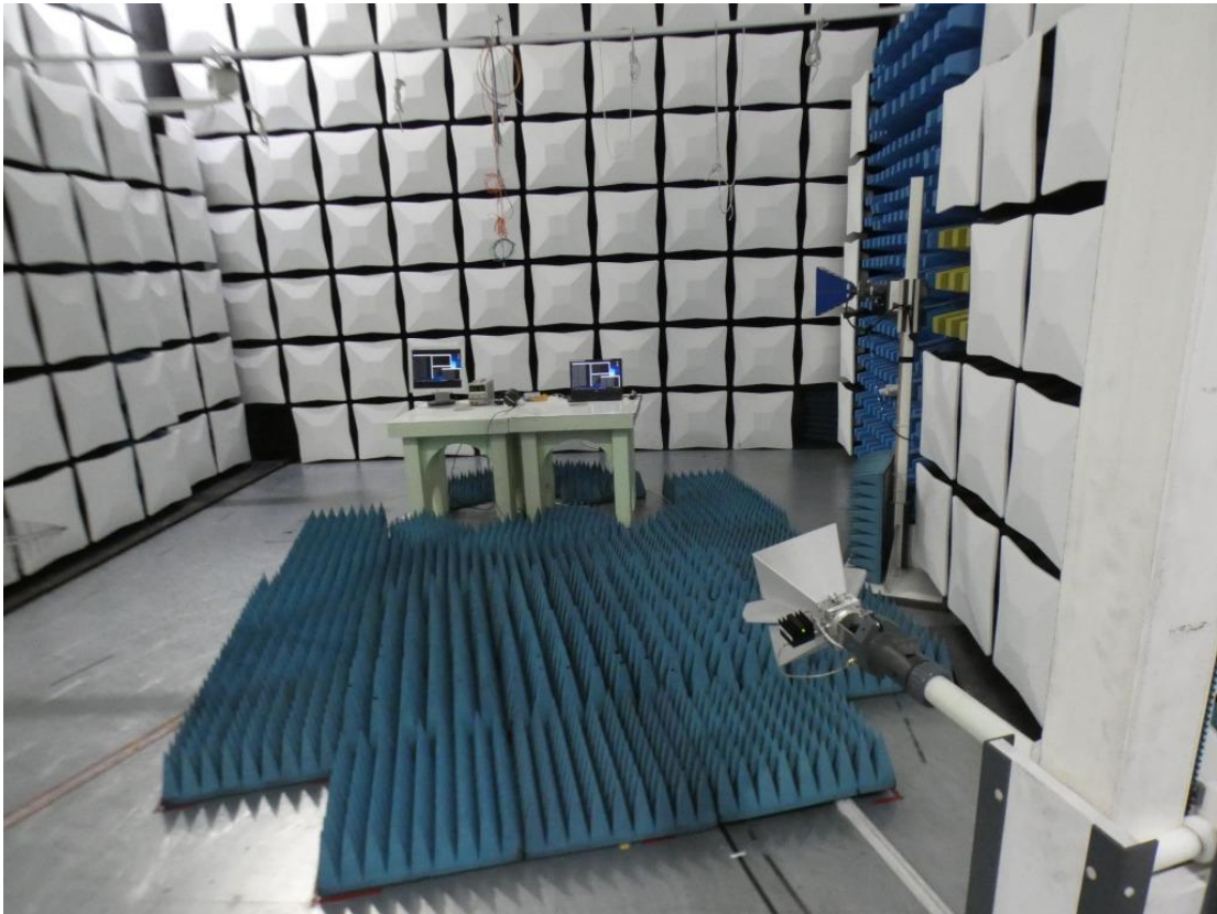
Photo 2: Test setup for radiated measurements FCC15b, above 1 GHz
