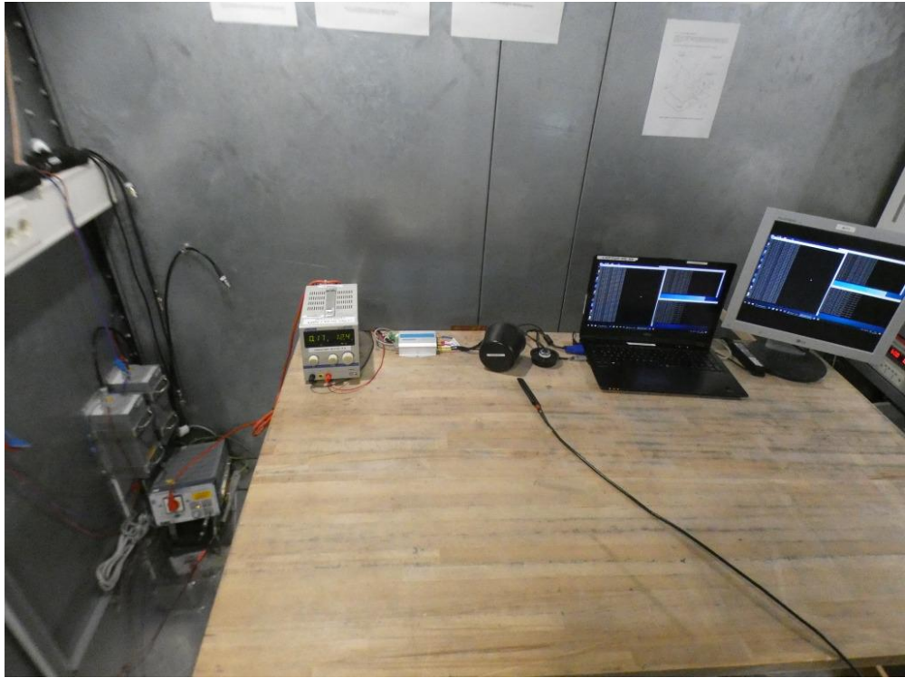
Photo 4: Test setup for conducted measurements FCC15b.
