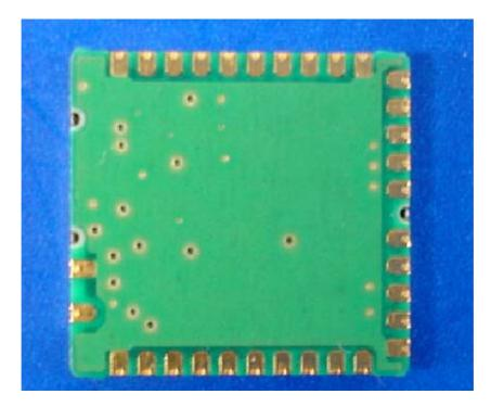
Photo without shielded case. Module with integral antenna and without.
