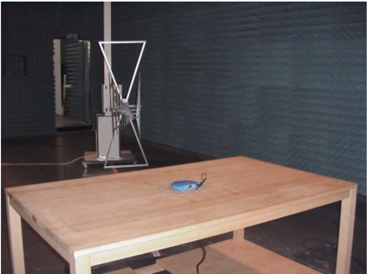
radiated measurements - test setup
