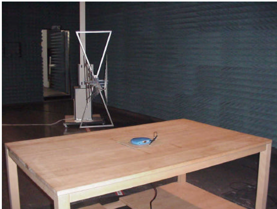
Picture 4 : Setup for radiated tests
