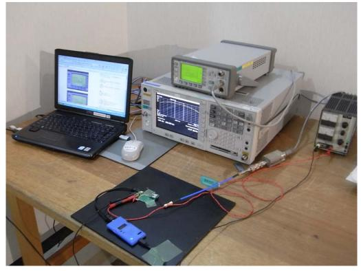
Transmitter Radiated Spurious Emissions (RF Radiated test)
